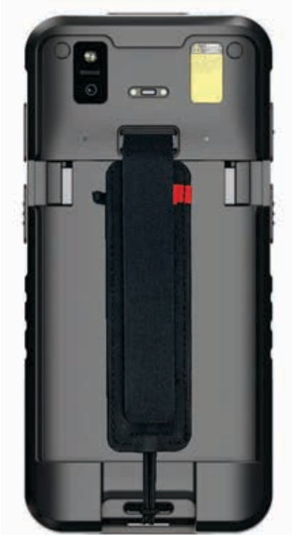
Standard Battery and Handstrap
