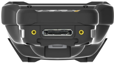
No I/O Cover installed
