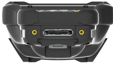
No I/O Cover installed
