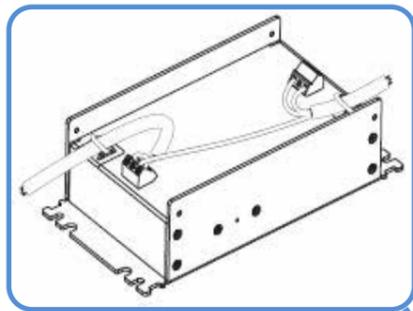
DC Converter Wiring
